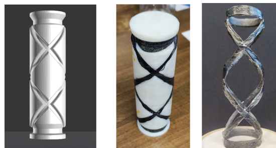
Figure 1: Left, Model of tool; Middle, Part layed up on HIPS tool; Right, Final part after removal of HIPS
