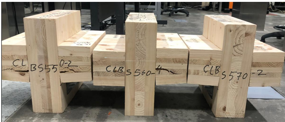
Figure 1: Specimens after compression test using TTP200 angle brackets and 3 screw lengths
