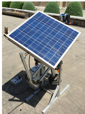
Figure 1: (a) Fabricated view of the solar tracker (b) Experimental and simulation results for generated power in a day by solar tracker compared with a fixed panel
